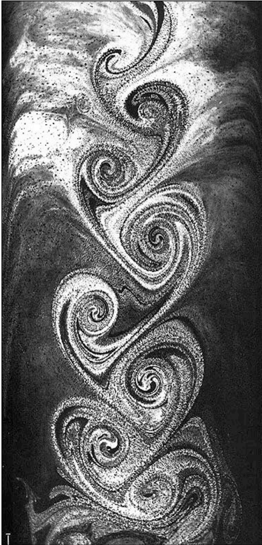
Figure 4. Karman Vortex Street behind a stick (Schwenk 1976)
